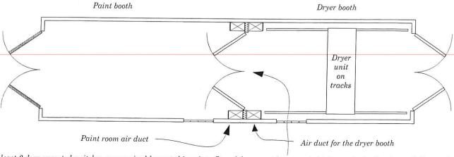
At least 2 door operated switches are required here at this point. One of these must be connected into a valve in the air supply line so that painting cannot take place until these doors are fully closed and the ventilating system is in full operation. The other door operated switch is required here to disallow operation of the dryer until these doors are fully closed and the ventilation system is in full operation
